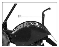
Fig. 2-10: Adjust Depth Regulator Lever.
